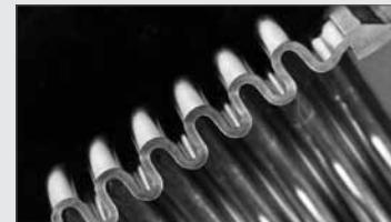
Fig. 3.18 Multi-ply bellows (section)
