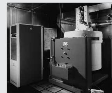
*Fig. 2.5 Vibration test stand for simulation of complex application conditions*
