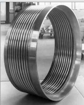
Fig. 8.6 Axial expansion joint made of Incoloy 825 for heat exchanger (DN 1200/PN 40)
