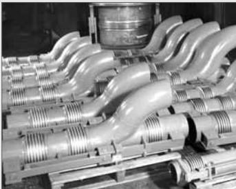
Fig. 8.2 Pressure balanced expansion joint
