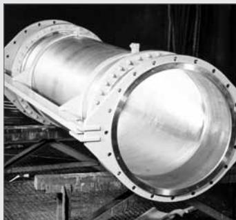
Fig. 8.25 HYDRAFLON lateral expansion joint for paper machines
