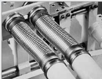
Fig. 2.6 Alternating bending apparatus for determination of the fatigue behaviour (service life provisions) of thin strips and metal sheets
