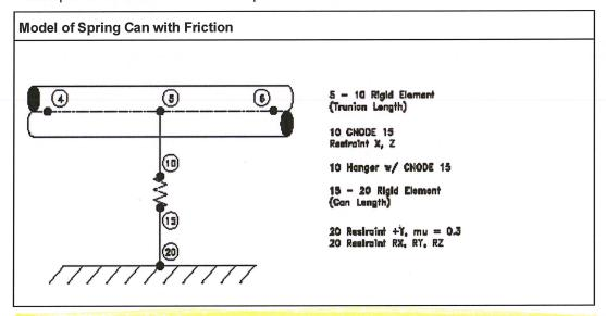
Alternatively, element 15-20 can be omitted with the +Y restraint (with friction) placed directly on node 15.
